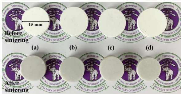
Figure 2. Appearance of the LD glass-ceramic samples with the powder-to-binder ratio of: a) 60:40, b) 55:45, c) 50:50, and d) 45:55 (vol.%) before and after sintering at 800 °C for 2 h
